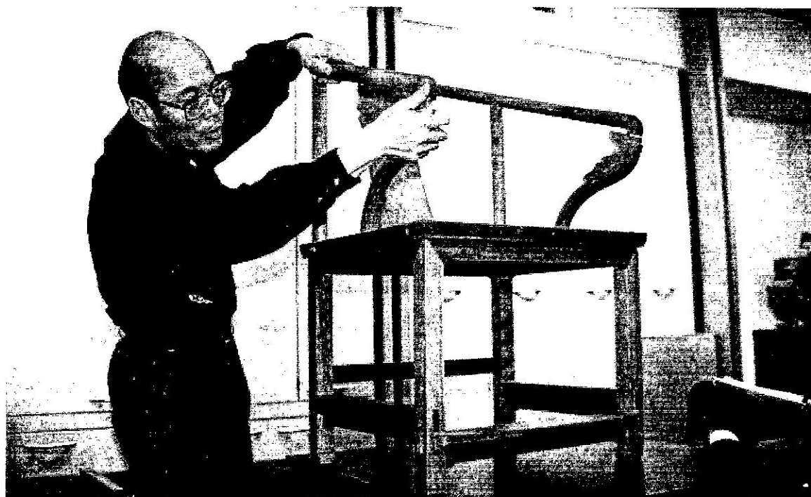
The final assembly of the chair. Note the structural yet decorative flat supports he's inserting under the front of the arms.
