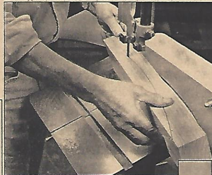
Tilting the bandsaw table and sawing a curve on the edge of the stock (above) produces the subtle arch in the lower rail of a chair (right).
